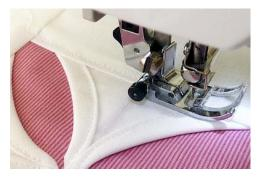
Attach first the 2" white strips to all four sides of your windows. After they are all on and ironed open, neatly top stitch about 1/8" from the edge. Since the windows are so thick and heavy, the sides can use a little help to lay flat once stuffed.
